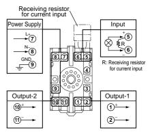
External receiving resistor for current input:
